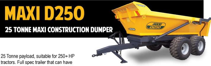
25 Tonne payload, suitable for 250+ HP tractors. Full spec trailer that can have options fitted. With large capacity and 12mm wearplate floor this dupmer has it all for the heavy construction scene.
