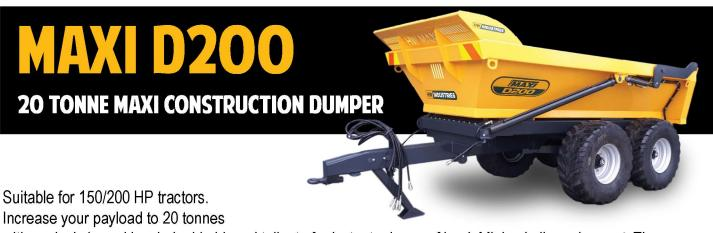
with conical shaped bowl, double hinged tailgate for instant release of load. Minimal oil requirement. The RTRA\* axles help make these the easiest trailers to pull through soft ground and are easy on the tyres on hard surfaces.
