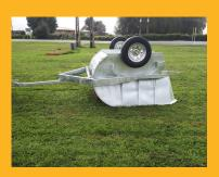
Holds 1.5m³ and size is suitable to be towed by quads, small & medium tractors, utes etc...
