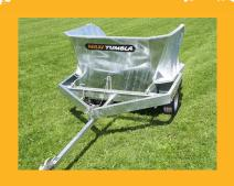
This size model suits the bigger ride ons, quads and small tractors. It holds  $1 \, \text{m}^3$  and is easily loaded over the sides. Has a easily accessible trip handle to activate the action of the rollover function to discharge the material in the bowl.
