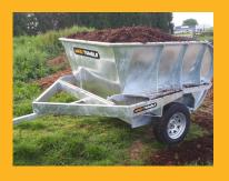
The large model is the biggest in our range and holds 2m<sup>3</sup>, it has all the features of the other models and is most suitable to be towed by utes and tractors.
